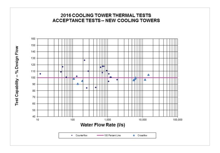
CTI tests are conducted by licensed agents that have been vetted to ensure that there is no conflict of interest. The licensed agent also has to have accurate code-compliant test instrumentation, detailed calibration records, years of testing experience, etc.
