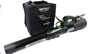
Sampler - Handheld device with a high-volume vacuum sampling fan and total flow rate monitor
