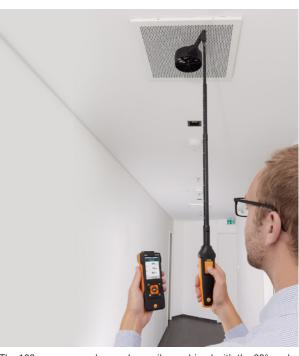
The 100 mm vane probe can be easily combined with the 90° angle and telescope, making measurements at ceiling outlets easier.
