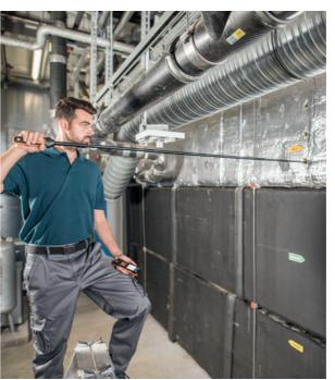
All testo 440 air velocity probes for measurements in ducts have a scaled, extendable telescope (optionally extendible from 1 to 2 m).
